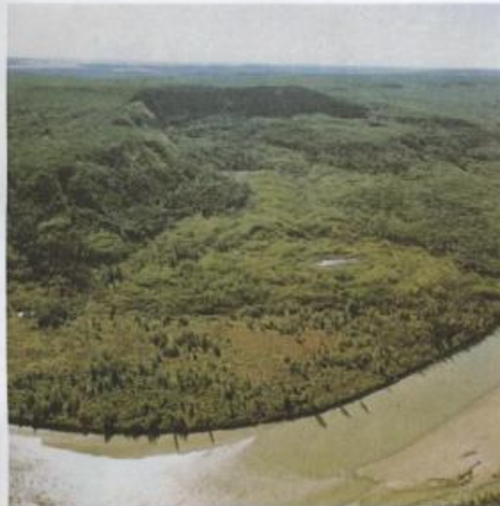
PHOTO 6-8. Looking southward over the Pine River toward a large slide in bedrock approximately one mile across. The slide occurred in shale of the Shaftesbury Formation. A similar slide 1.5 miles across and 1500 feet high occurred on the north bank of the Peace River downstream of Cache Creek.
